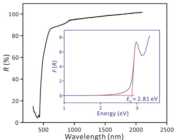
Fig. 3 UV-vis-NIR transmittance spectrum of  $\text{Cs}_3\text{VO}(\text{O}_2)_2\text{CO}_3$ . The inset shows an optical diffuse reflectance spectrum of  $\text{Cs}_3\text{VO}(\text{O}_2)_2\text{CO}_3$ .
