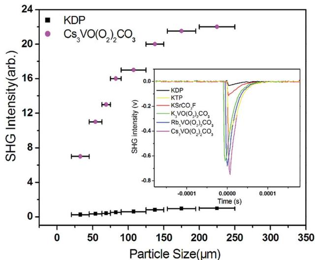
Fig. 4 Phase-matching curve for  $\text{Cs}_3\text{VO}(\text{O}_2)_2\text{CO}_3$ . The inset reveals oscilloscope traces showing the SHG intensity for  $\text{A}_3\text{VO}(\text{O}_2)_2\text{CO}_3$  (A = K, Rb, and Cs). The SHG intensities for KDP, KTP, and  $\text{K SrCO}_3\text{F}$  are also plotted for comparison.
