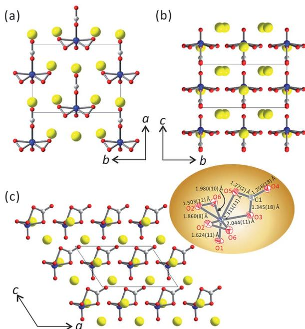
Fig. 1 Ball-and-stick models of  $\text{Cs}_3\text{VO}(\text{O}_2)_2\text{CO}_3$  in the (a)  $ab$  plane, (b)  $bc$  plane, and (c)  $ac$  plane (yellow, Cs; blue, V; gray, C; and red, O). The  $[\text{VO}(\text{O}_2)_2\text{CO}_3]$  units align parallel to  $\text{CO}_3$  groups and orient in the same direction.
