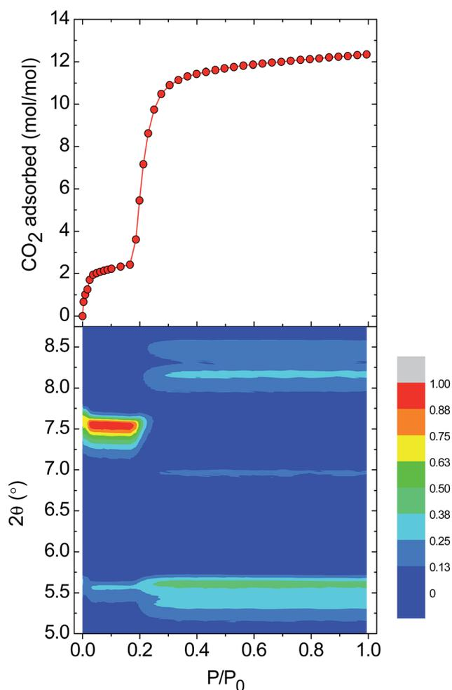
Fig. 4 (top) The adsorption branch of the CO<sub>2</sub> uptake measurements performed at 195 K on **1-a**. (bottom) A contour plot of the evolution of the Bragg peaks over the range  $2\theta = 5.0$ – $8.75^\circ$  as a function of  $P/P_0$ . The intensity of the peaks is relative to the strong peak observed at  $7.54^\circ$  over the pressure range  $P/P_0 = 0.035$ – $0.18$ .
