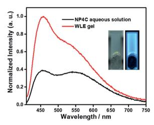
Fig. 7 PL emission spectra of the WLE hydrogel ( $\sim$ 2 wt%) and its adopted NP4C aqueous solution excited at 400 nm, [NP4C] = 0.1 mM, and 25 °C. Inset: photographs of the WLE hydrogel in daylight and 365 nm UV light, respectively.
