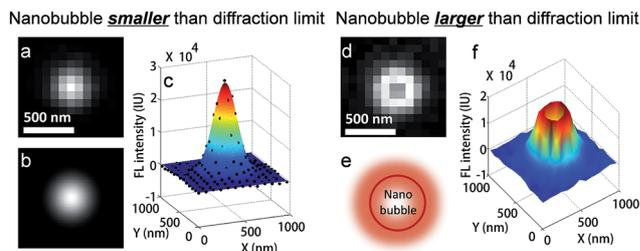
Fig. 2 FL images of H<sub>2</sub> nanobubbles generated at single CdS NPs during photocatalysis. Experimental (a) and fitted (b, c) FL images of a single nanobubble smaller than the diffraction limit. For nanobubbles larger than the diffraction limit, the FL image shows a ring-shaped pattern in the 2-dimensional (d) and 3-dimensional (f) views because R6G molecules are adsorbed at the surface of the nanobubble (e).
