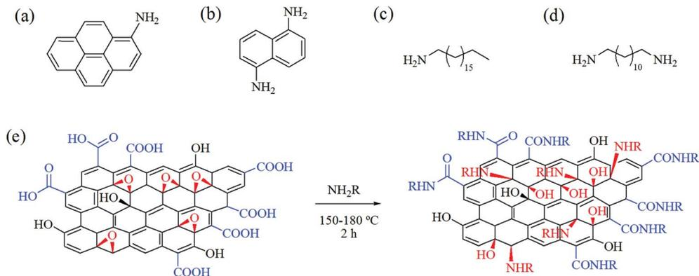
**Fig. 1** Chemical structures of amines employed in the present study: (a) 1-aminopyrene, (b) 1,5-diaminonaphthalene, (c) 1-octadecylamine and (d) 1,12-diaminododecane. (e) Suggested general scheme for the transformation of GOP functional groups (carboxylic, in blue; epoxy, in red) upon functionalization with amines. R = aryl or alkyl.
