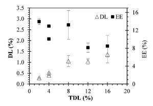
Fig. 3 Drug loading ( $\Delta$ ) and encapsulation efficiency ( $\blacksquare$ ) for the MB-PNP with different theoretical drug loading experiments prepared by the different emulsification techniques. Data represent mean (n = 3).
