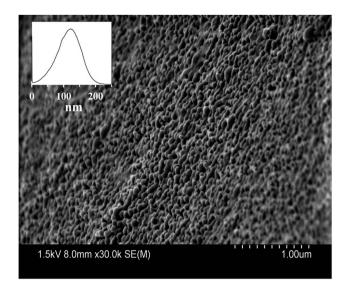
Fig. 4 Scanning electron micrograph of blank-PNP. The insert represents the particle size distribution histogram of blank-PNP.
