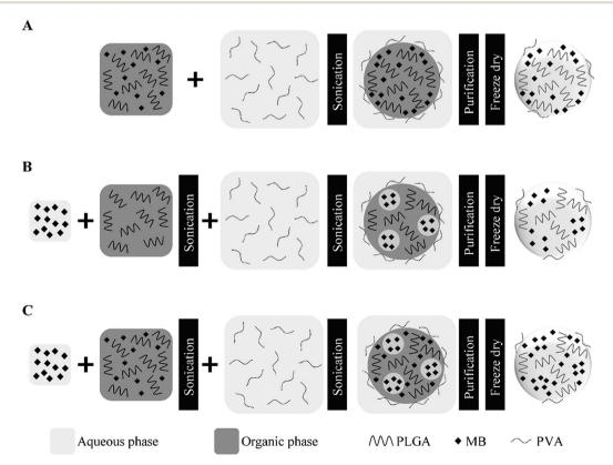
Fig. 1 Schematic of MB loaded PLGA nanoparticle preparation. Single (A), double (B) and combined (C) emulsification techniques.
