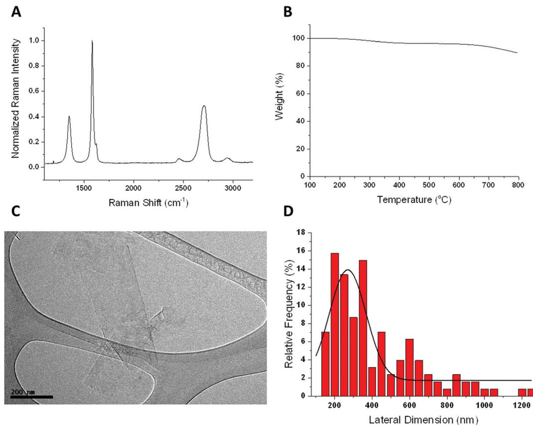
**Fig. 1** Chemical characterization of FLG by Raman spectroscopy as an average of 28 spectra (A), thermogravimetric analysis (B), representative HRTEM image (C) and lateral size distribution ( $n = 107$ ) of FLG (D).
