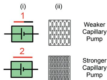
Fig. 6 (i) Symbolic and (ii) schematic representation of capillary pump. The spacing between microstructures in the pump determines its capillary pressure. Stronger capillary pumps have more closely spaced microstructures.
