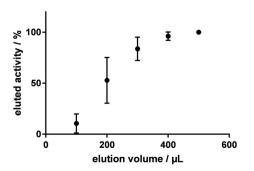
Fig. 1 Elution efficiency of 0.1 M K<sub>2</sub>SO<sub>4</sub> in water.
