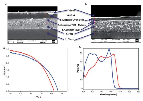
Fig. 9 SEM cross-sectional image of (a) (BdA)Pb<sub>2</sub>I<sub>6</sub> and (b) (BdA)PbI<sub>4</sub> based solid-state solar cells showing their related architectures. Obtained (c) current-voltage and (d) IPCE curves of --- (BdA)Pb2l6 and --- (BdA)Pb14 solar cells. A mesoporous TiO2 layer was used as the electron transporting material and gold was used as the back contact.
