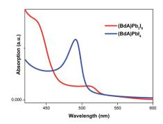
Fig. 4 Absorption spectra of spincoated --- 1D and --- 2D butyl-1,4-diammonium lead( $\shortparallel$ ) iodide materials on TiO<sub>2</sub> films. A small red shift in the band edge is observed for the one-dimensional (BdA)Pb<sub>2</sub>I<sub>6</sub> as compared to two-dimensional (BdA)PbI<sub>4</sub>, 544 nm and 523 nm, respectively.
