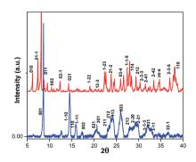
Fig. 3 Powder diffraction patterns for the --- (BdA)Pb1 $_4$  and --- (BdA) Pb $_2$ I $_6$ . Miller indices were obtained from single crystal data.
