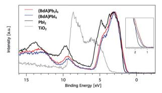
Fig. 6 Valence levels of the TiO<sub>2</sub> film, TiO<sub>2</sub>/PbI<sub>2</sub> and (BdA)Pb<sub>2</sub>I<sub>6</sub> and (BdA)Pbl<sub>4</sub> measured with a photon energy of 4000 eV. A valence band edge shift was observed for --- (BdA)Pb<sub>2</sub>I<sub>6</sub> when compared to --- (BdA) Pbl₄.
