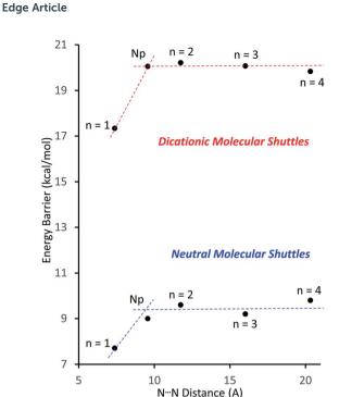
Fig. 4 Plots of the energy barrier to translational motion in the molecular shuttles *versus* the distance between N-atoms on opposite ends of the track. Dotted lines are for visualisation purposes only (n = number of phenyl rings, Np = naphthyl).
