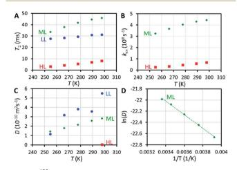
Fig. 3 (A)  $^{129}$ Xe  $T_2$  relaxation times of xenon in CC3-R as a function of temperature. (B) Rates of xenon exchange between the window and cage cavities extracted from  $T_2$  data. (C) Diffusion coefficient of xenon in CC3-R as a function of temperature. The data of the LL sample is scattered because of the low signal-to-noise ratio in the experiment due to the low xenon concentration in the sample. (D) Arrhenius plot of the ML sample.
