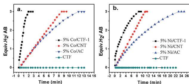
Fig. 3 Plots of volume of H<sub>2</sub> generated *vs.* time for AB hydrolysis catalyzed by (a) 5% Co/CTF-1, 5% Co/CNT, 5% Co/AC, CTF (b) 5% Ni/CTF-1, 5% Ni/CNT, 5% Ni/AC, CTF. ([AB] = 322 mM, 5 mL,  $n_{\text{metal}}/n_{\text{AB}} = 0.05$ ).
