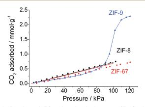
Fig. 2 Experimental  $CO_2$  adsorption isotherms at 25 °C of the powdered cobalt-based materials ZIF-9 (blue triangles) and ZIF-67 (red circles), compared with the ZIF-8  $CO_2$  isotherm (black squares) reported by Zornoza *et al.*<sup>56</sup> Solid lines show simulated ZIF-8 (black) and ZIF-67 (red) isotherms with a good fit to the experimental data (filled symbols). The solid line in the ZIF-9 isotherm is a guide to the eye.
