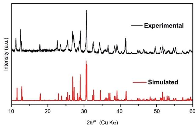
Fig. 1 Experimental and simulated powder X-ray diffraction patterns of the Na<sub>2</sub>Tb<sub>1.08</sub>Ca<sub>2.92</sub>Si<sub>6</sub>O<sub>18</sub>H<sub>0.8</sub> compound. The simulated pattern is based on the structure refined by our single-crystal X-ray diffraction analysis.
