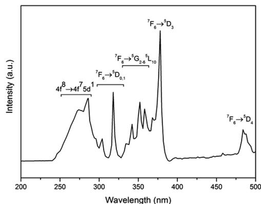
Fig. 3 Excitation spectrum of  $\text{Na}_2\text{Tb}_{1.08}\text{Ca}_{2.92}\text{Si}_6\text{O}_{18}\text{H}_{0.8}$  ( $\lambda_{\text{em}} = 542$  nm).
