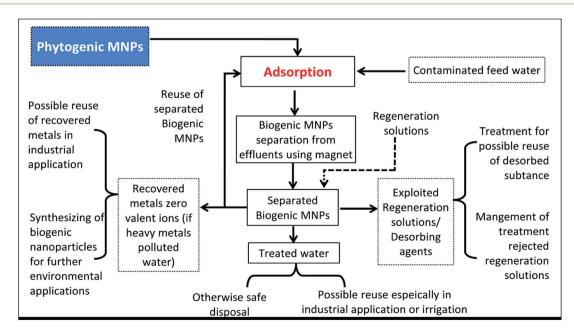
Fig. 10 Schematic of our proposed phytogenic magnetic nanoparticles (PMNPs) based zero effluent discharge water/wastewater treatment (WWT) process.
