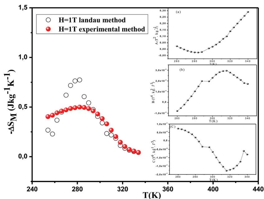
**Fig. 3** Experimental and calculated values of the magnetic entropy change vs. temperature used the Landau theory under applied magnetic field of 1 T for the  $\text{La}_{0.7}\text{Ca}_{0.1}\text{Pb}_{0.2}\text{Mn}_{0.9}\text{Al}_{0.05}\text{Sn}_{0.05}\text{O}_3$  compound. The inset: (a)–(c): variation of Landau parameters  $A$ ,  $B$  and  $C$  as a function of temperature of  $\text{La}_{0.7}\text{Ca}_{0.1}\text{Pb}_{0.2}\text{Mn}_{0.9}\text{Al}_{0.05}\text{Sn}_{0.05}\text{O}_3$ .
