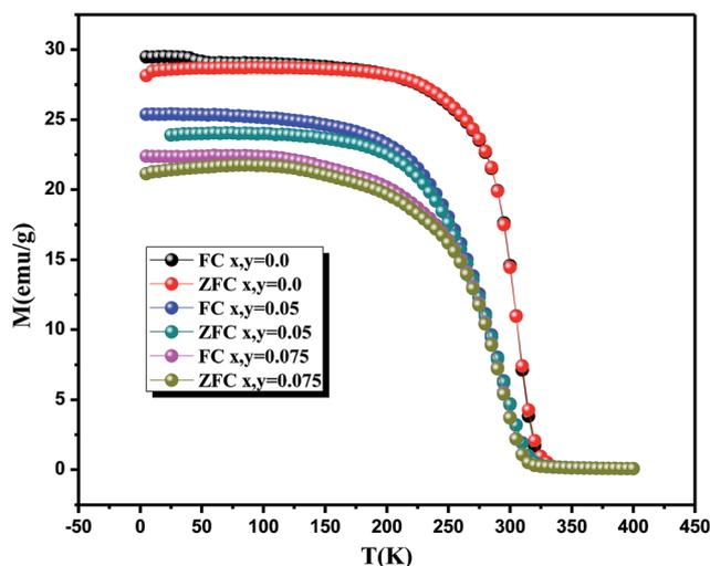
Fig. 1 Temperature dependences of ZFC and FC magnetization for  $\text{La}_{0.7}\text{Ca}_{0.1}\text{Pb}_{0.2}\text{Mn}_{1-x-y}\text{Al}_x\text{Sn}_y\text{O}_3$  ( $x, y = 0.0, 0.05$  and  $0.075$ ) compounds under a magnetic field of 0.05 T.
