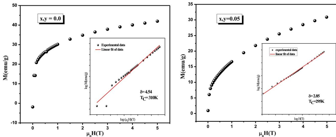
Fig. 10 Critical isotherms of  $M$  versus  $\mu_0 H$  for  $\text{La}_{0.7}\text{Ca}_{0.1}\text{Pb}_{0.2}\text{Mn}_{1-x-y}\text{Al}_x\text{Sn}_y\text{O}_3$  ( $x, y = 0.0$  and  $0.05$ ). The inset: shows the log–log scale for  $M$  versus  $\mu_0 H$ .
