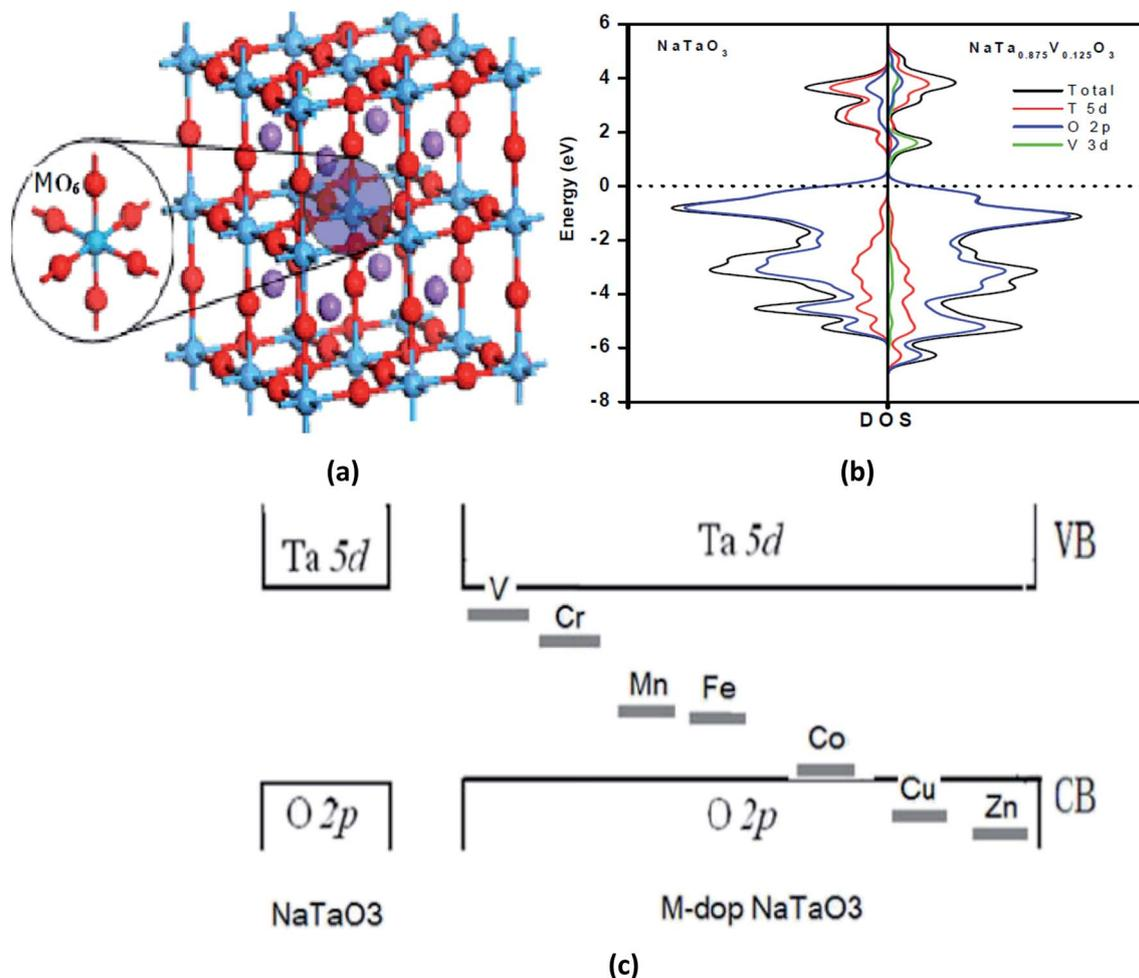
Fig. 6 (a) A supercell of M-doped  $\text{NaTaO}_3$   $2 \times 2 \times 2$  (40-atoms), (b) the total density of states and projected density of states of the pure and V-doped  $\text{NaTaO}_3$ , and (c) intermediate band formation by the d-orbital of the doped metal ions. Reprinted with permission of ref. 184. Copyright 2012 IACSIT Press, Singapore.
