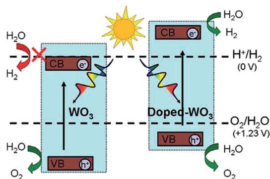
Fig. 5 A schematic of the superior photocatalytic activity of metal-doped  $\text{WO}_3$  for  $\text{H}_2$  production as compared to that of  $\text{WO}_3$ . Reprinted with permission of ref. 179. Copyright 2012 American Chemical Society.
