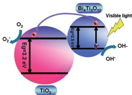
Fig. 3 A schematic showing the energy band structure and electron-hole pair separation in the  $\text{Bi}_4\text{Ti}_3\text{O}_{12}/\text{TiO}_2$  heterostructure. Reprinted with permission of ref. 124. Copyright 2011 Royal Society of Chemistry.
