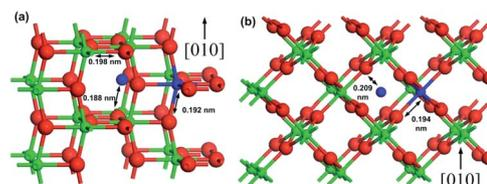
**Fig. 2** A schematic of the interstitial and substitutional dopant positions in (a) anatase and (b) rutile  $\text{TiO}_2$  with the arrows showing the cation-dopant to oxygen distances. Reprinted with permission of ref. 100. Copyright 2012 Springer-Verlag Berlin Heidelberg.
