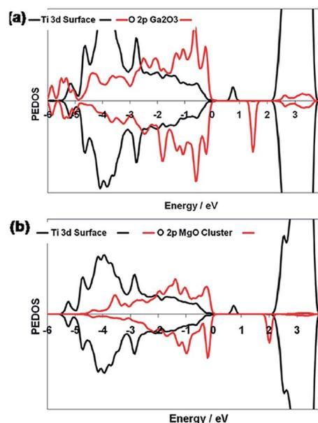
Fig. 4 Ti 3d and O 2p PEDOS of the  $(\text{Ga}_2\text{O}_3)_2$  and  $(\text{MgO})_4$  clusters for the relaxed triplet excited states of (a)  $\text{Ga}_2\text{O}_3$ -modified  $\text{TiO}_2$  and (b)  $\text{MgO}$ -modified  $\text{TiO}_2$ . The zero of energy is the top of the valence band. Reprinted with permission of ref. 134. Copyright 2012 American Chemical Society.
