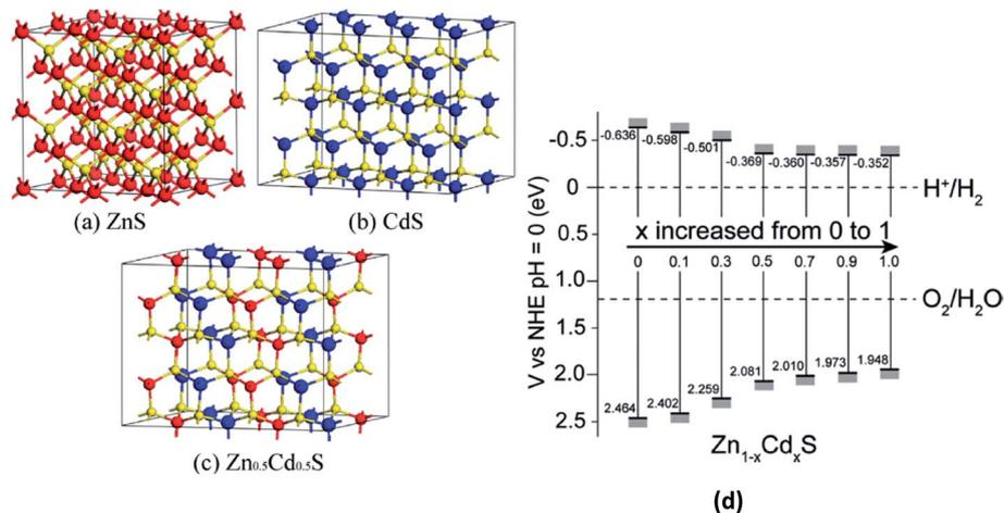
Fig. 8 The supercell models for bulk (a) ZnS (64 atoms) and (b) CdS (64 atoms). The red, yellow, and blue spheres represent the Zn, S, and Cd atoms, respectively. (c) The geometry model for  $Zn_{0.5}Cd_{0.5}S$  and (d) conduction and valence band edge potentials of the  $Zn_{1-x}Cd_xS$  samples ( $x = 0, 0.1, 0.3, 0.5, 0.7, 0.9, \text{ and } 1.0$ ). Reprinted with permission of ref. 223. Copyright 2013 American Chemical Society.
