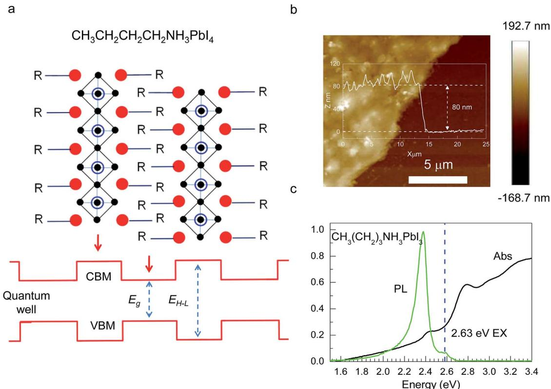
Fig. 1 (a) Schematic illustration of 2D layered  $\text{CH}_3\text{CH}_2\text{CH}_2\text{CH}_2\text{NH}_3\text{PbI}_4$  perovskite and its quantum-well electronic structures. (b) AFM image of a  $\text{CH}_3\text{CH}_2\text{CH}_2\text{CH}_2\text{NH}_3\text{PbI}_4$  perovskite film spin coated on quartz. (c) Absorption and photoluminescence spectra of the 2D perovskite at room temperature.
