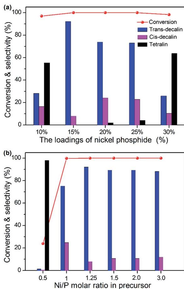
Fig. 6 Naphthalene conversion and selectivity to decalin (a) over  $\text{Ni}_x\text{P-Al-M}$  with different  $\text{Ni}_x\text{P}$  loadings and (b) over  $\text{Ni}_x\text{P-Al-M}$  with different Ni/P molar ratio in precursor as 0.5, 1.0, 1.25, 1.5, 2.0, and 3.0 at  $270 \text{ }^\circ\text{C}$  and 3 MPa.
