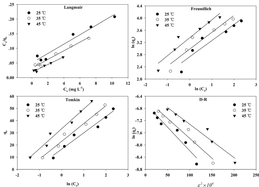
Fig. 9 The fitting of Langmuir, Freundlich, Temkin, D–R isotherms for Cr(vi) adsorption onto the TW/Fe<sub>3</sub>O<sub>4</sub> composite.
