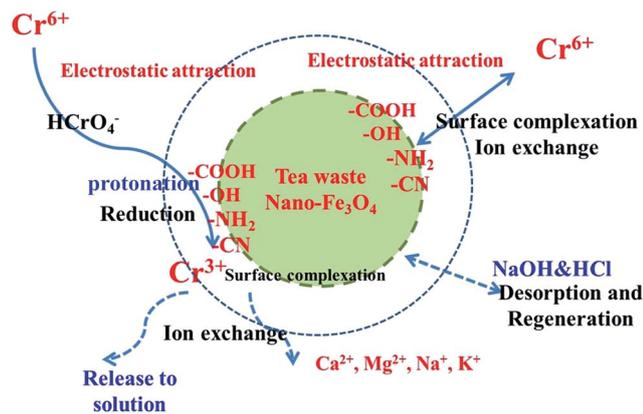
Fig. 14 Proposed mechanism of Cr(vi) removal by the TW/Fe<sub>3</sub>O<sub>4</sub> composite.
