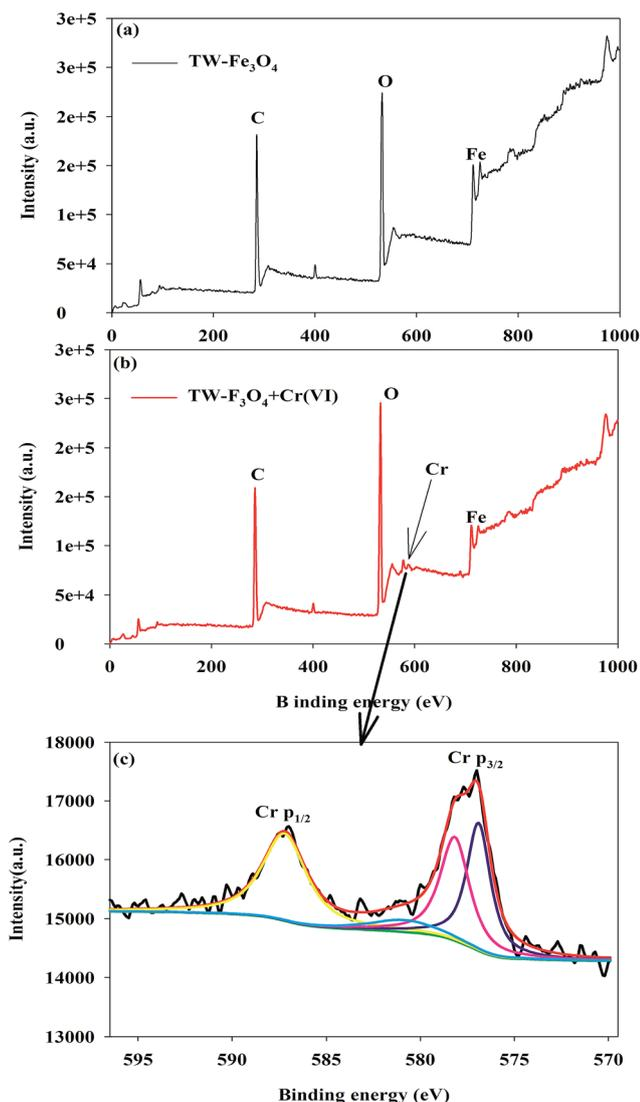
Fig. 5 XPS analysis of the TW/Fe<sub>3</sub>O<sub>4</sub> composite and adsorbed Cr on the TW/Fe<sub>3</sub>O<sub>4</sub> composite (a) TW/Fe<sub>3</sub>O<sub>4</sub> composite (b) Cr laden on the TW/Fe<sub>3</sub>O<sub>4</sub> composite (c) speciation analysis of Cr.
