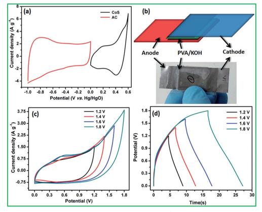
Fig. 7 (a) CV profile of the positive and negative electrodes at a scan rate of 30 mV s<sup>-1</sup>. (b) Image of the fabricated all-solid-state asymmetric supercapacitor device. (c) CV profile of the asymmetric cell at different cell voltages. (d) CD profile of the asymmetric cell at different cell voltages.
