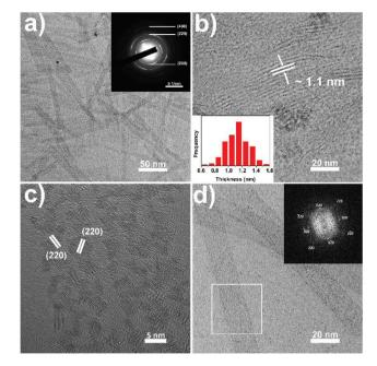
Fig. 3 Characterization of the as-synthesized ceria SL-nanoplates. (a, b) TEM images; (c) HRTEM image; (d) TEM images; the inset in (a) is the SAED pattern of the ceria SL-nanoplates; the inset in (b) shows the thickness distribution of the SL-nanoplates; the inset in (d) is the FFT pattern of the selected area in (d).
