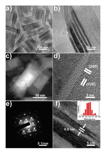
Fig. 4 Characterization of the as-synthesized ceria ML-nanoplates. (a, b) TEM images; (c) HAADF-STEM image; (e) SAED pattern; (d, f) HRTEM images; the inset in (f) shows the thickness distribution of the layers in the ML nanoplates.
