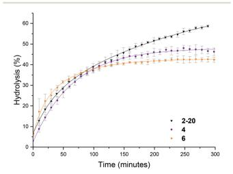
Fig. 6 Hydrolysis kinetics of short, medium and long armed PEGA stars (2-20, 4, and 6 respectively), at 50  $^{\circ}$ C in  $D_2$ O as determined by  $^{1}$ H NMR spectroscopy. Error bars produced from the standard deviation of 3 repeats.
