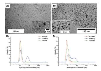
Fig. 3 Representative TEM images and size distributions, as determined by DLS (5 mg mL<sup>-1</sup> in chloroform), of PEGA<sub>98</sub>-b-(DMAEA<sub>76</sub>-co-DEGDA<sub>16</sub>), 2-20 (a and c), and PEGA<sub>98</sub>-b-(DMAEA<sub>72</sub>-co-DEGDA<sub>8</sub>), 2-10 (b and d) prepared by arm-first RAFT polymerization.
