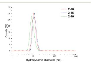
Fig. 2 Size distributions, by number, for PEGA armed particles 2-20, **2-15**, **2-10**, obtained by DLS (detection angle =  $173^{\circ}$ ) at 5 mg mL<sup>-1</sup> carried out in chloroform at 25 °C.
