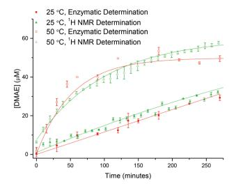
Fig. 10 Comparison between the theoretical concentration of DMAE released based on <sup>1</sup>H NMR spectroscopic analysis (green) and enzymatically determined (red) at 25 and 50 °C. Error bars produced from the standard deviation of three repeats.
