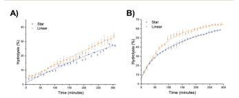
Fig. 7 Hydrolysis kinetics of 2-20 and the linear analogue PEGA<sub>98</sub>-b-(DMAEA $_{60}$ -co-MA $_{13}$ ) at (a) 25 °C and (b) 50 °C, in D $_2$ O as determined by <sup>1</sup>H NMR spectroscopy. Error bars produced from the standard deviation of 3 repeats.
