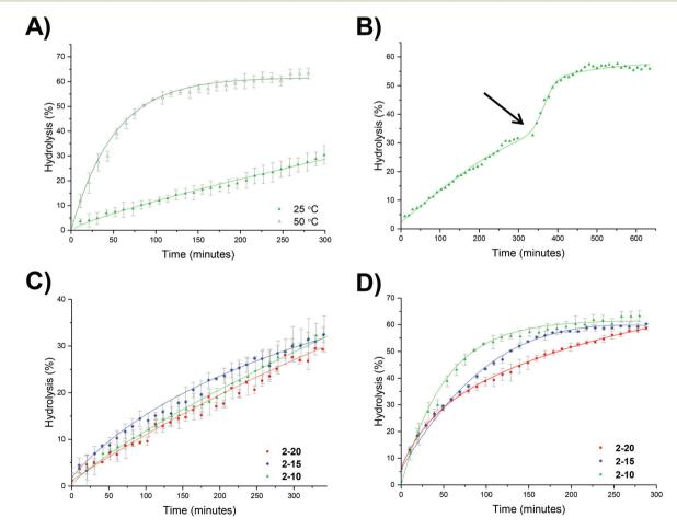
Fig. 5 Hydrolysis kinetics of PEGA-b-(DMAEA-co-DEGDA) in D<sub>2</sub>O as determined by <sup>1</sup>H NMR spectroscopy: (a) hydrolysis of **2-10** carried out at 25 °C and 50 °C; (b) 2-10 initially heated at 25 °C with an increase in temperature to 50 °C at 320 minutes; (c) hydrolysis at 25 °C with different crosslinking densities, and (d) hydrolysis at 50 °C with different crosslinking densities. Error bars produced from the standard deviation of 3 repeats.
