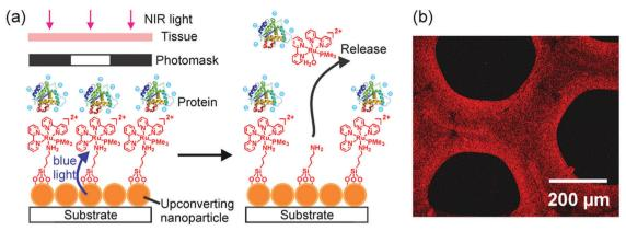
Fig. 11 (a) Schematic of photon upconversion lithography for the patterning of proteins. Polyethylene glycol, which is co-grafted with Ru complexes on the UCNPs, is not shown for clarity. (b) Confocal laser scanning microscopy image of a protein pattern fabricated using photon upconversion lithography. Adapted with permission. 81 Copyright 2015, Wiley-VCH Verlag GmbH & Co. KGaA.
