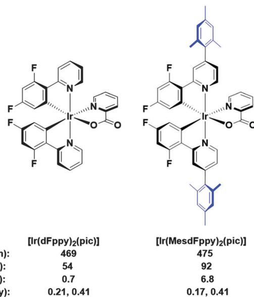
Fig. 2 FIrpic and its mesityl functionalised analogue. The mesityl functionality confers improved properties in virtually all important metrics, including solution state  $\Phi_{\text{PL}}$ , as well as  $\eta_{\text{ext}}$  values and CIE coordinates for comparable solution processed device architectures. This comes only at the expense of a small red-shift in solution state  $\lambda_{\text{max}}$ .
