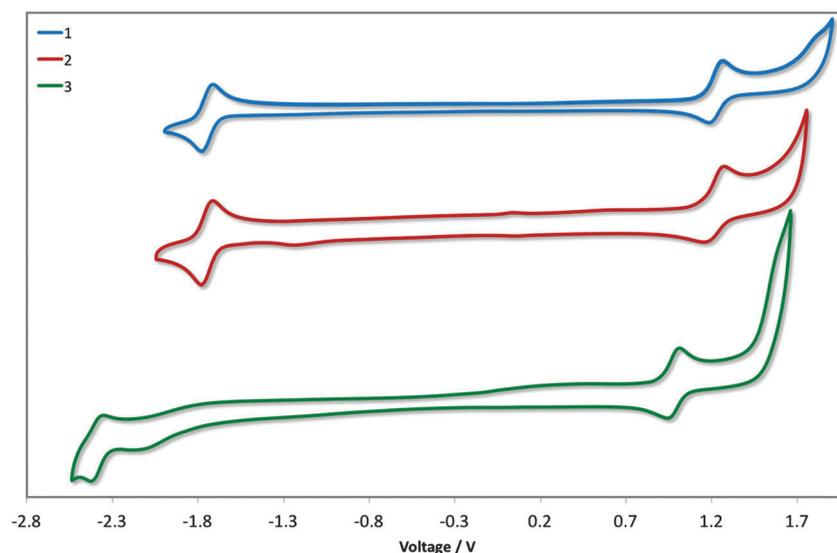
Fig. 6 CV traces of complexes **1–3** in MeCN solution, reported versus SCE (Fc/Fc<sup>+</sup> = 0.38 V in MeCN)<sup>22</sup> redox couple. Scan rates were at 100 mV s<sup>−1</sup>, and are in the positive scan direction.
