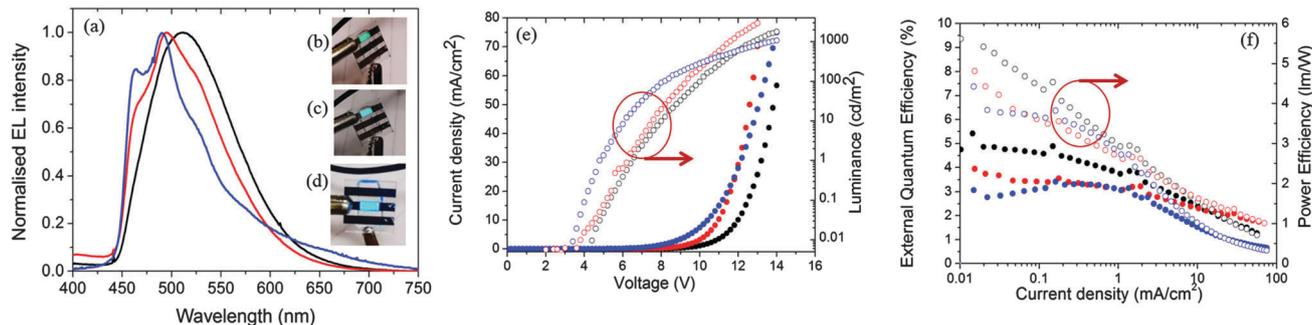
**Fig. 11** (a) Normalized electroluminescent emission spectra of **1** (black), **2** (red) and **3** (blue) in thin films. Photograph of the working OLED with (b) **1** (c) **2** and (d) **3**. (e) Current density and luminance versus applied voltage for OLEDs. (f) External quantum efficiency (solid circles) and power efficiency (open circles) versus applied voltage for OLEDs made with **1** (black) and **2** (red) and **3** (blue).
