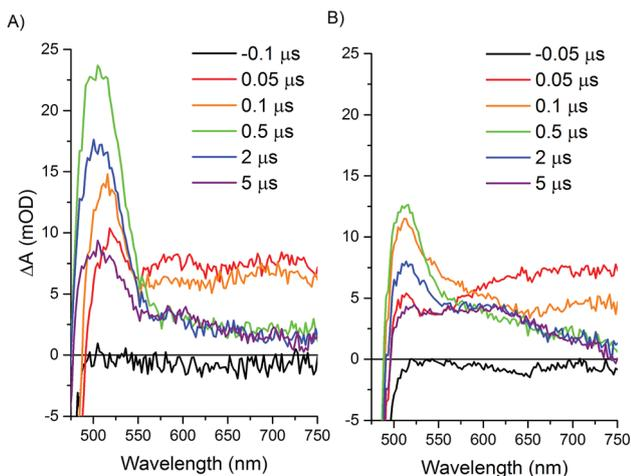
Fig. 5 Transient optical absorption spectra at selected early times. Samples contained 200 mM sodium ascorbate and were excited at 460 nm and detected with a fiber laser. (A) Ru-ApoFld-CoBF<sub>2</sub> spectra, (B) Ru-Fd-CoBF<sub>2</sub> spectra.
