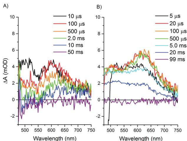
**Fig. 7** Transient optical absorption spectra at selected later times. Samples contained 200 mM sodium ascorbate and were excited at 460 nm and detected with a fiber laser. (A) Ru–ApoFld–CoBF<sub>2</sub> spectra, (B) Ru–Fd–CoBF<sub>2</sub> spectra.
