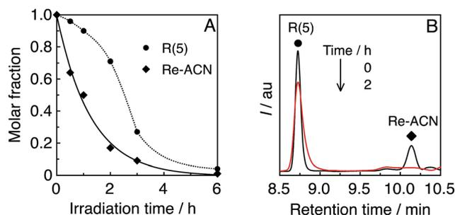
Fig. 6 (A) Residual **R(5)** and **Re-ACN** in solution during the photocatalytic reaction, obtained using UPLC analysis (Fig. S9, ESI†). (B) UPLC chart of the photocatalytic system **R(5)/Re-ACN** before and after 2 h of irradiation;  $\lambda_{\text{det}} = 350 \text{ nm}$ .
