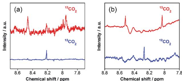
Fig. 7  $^1\text{H}$  NMR spectra of reaction solutions (2 mL) containing  $\text{RuRu}/\text{Ag}/\text{TaON}$  (8 mg) in (a)  $\text{H}_2\text{O}$ -MeOH (4 : 1 v/v) and (b)  $\text{H}_2\text{O}$ -iPrOH (4 : 1 v/v) after a 48 h irradiation with visible light ( $\lambda > 400$  nm) under  $^{13}\text{CO}_2$  (red) and  $^{12}\text{CO}_2$  (blue) atmospheres.
