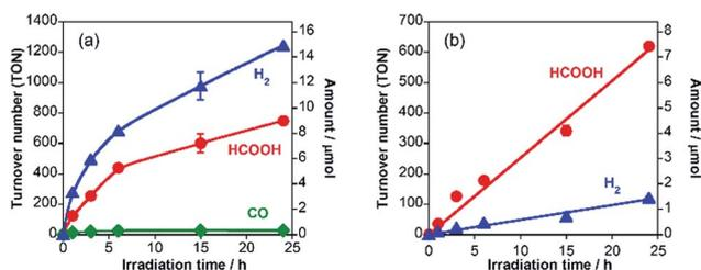
Fig. 2 Time courses of HCOOH (red),  $\text{H}_2$  (blue) and CO (green) formation by visible-light ( $\lambda > 400$  nm) irradiation to **RuRu**/Ag/TaON (4 mg) in  $\text{EDTA}\cdot 2\text{Na}$  (10 mM) aqueous solution (4 mL) without (a) and with (b)  $\text{Na}_2\text{CO}_3$  (0.1 M) under a  $\text{CO}_2$  atmosphere.
