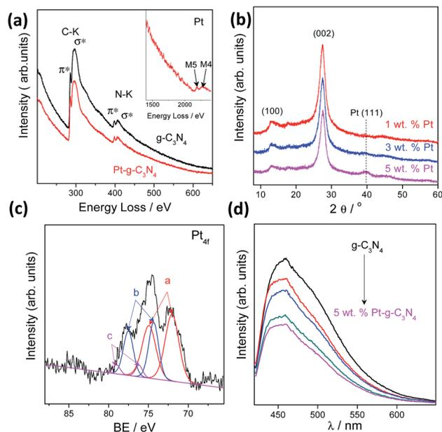
Fig. 3 (a) EELS of the g-C<sub>3</sub>N<sub>4</sub> polymers with Pt deposited *in situ*. (b) XRD of the g-C<sub>3</sub>N<sub>4</sub> polymers with Pt deposited *in situ*. (c) High resolution of XPS analysis of Pt<sub>4f</sub>. (d) PL spectra of the g-C<sub>3</sub>N<sub>4</sub> polymers with Pt deposited *in situ*.
