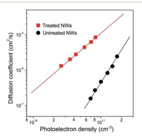
Fig. 2 Electron transport properties of NW arrays. Dependence of electron diffusion coefficients (D) on the photoelectron density (n) for untreated (black line) and treated (red line) NW arrays. The electron transport in NW arrays is found to be over 20-fold improved after the wet-chemistry treatment.
