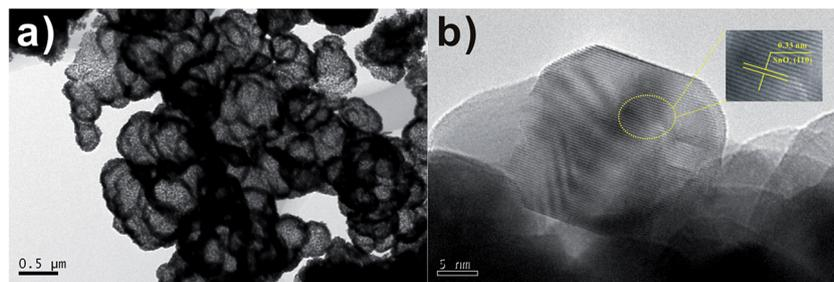
Fig. 4 (a) TEM (b) HRTEM images of SnO<sub>2</sub> samples after calcination at 550 °C for 3 h with 1 : 2 molar ratio of D-glucose and SnCl<sub>2</sub>·2H<sub>2</sub>O.
