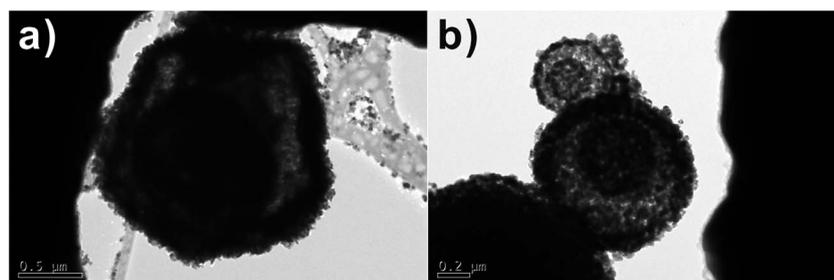
Fig. 7 TEM images of  $\text{SnO}_2$  samples after calcination at (a)  $700^\circ\text{C}$  and (b)  $500^\circ\text{C}$  with 1 : 1 molar ratio of sucrose and  $\text{SnCl}_4 \cdot 5\text{H}_2\text{O}$ .
