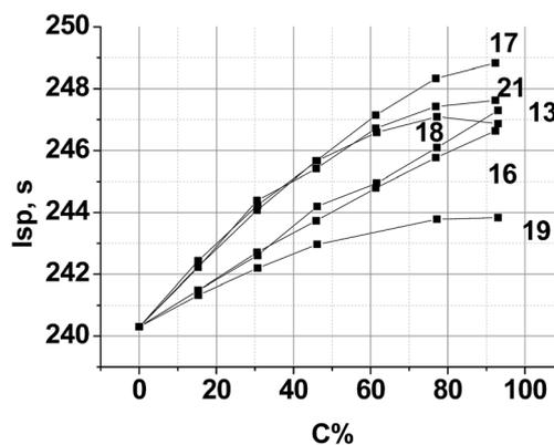
Fig. 7 Calculated specific impulse  $I_{sp}$  of (AP + new compound)–Al(20%)–AB(14–15%) propellants over various new compound loadings. Here, C is the percentage of a new compound in the mixture with AP.
