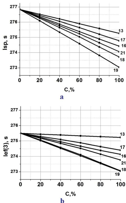
Fig. 8 (a) Calculated specific impulse  $I_{sp}$  of ADN(50%)–AlH<sub>3</sub>(25%)–PMVT(5%)–(NG + new compound) (20%) propellants over various new compound loadings. Here, C is the percentage of a new compound in the mixture with NG. (b)  $I_{ef}(3)$  characterized the ballistic effectiveness of the propellants utilized in the third stage of rocket complex,  $I_{ef}(3) = I_{sp} + 25 \times (\rho - 1.7)$ .<sup>48</sup> It is a relative effectiveness of propellants with different densities.
