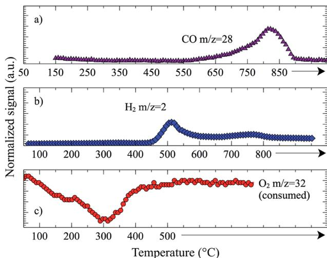
Fig. 8 Oxidation of  $\text{La}_{0.75}\text{Sr}_{0.25}\text{CoO}_3$  previously reduced with 10%  $\text{H}_2/\text{He}$  at 600 °C for 30 min (total flow rate 50 sccm). (a) Oxidation with  $\text{CO}_2$  forming CO. (b) Oxidation with  $\text{H}_2\text{O}$  forming  $\text{H}_2$ . (c) Consumption of  $\text{O}_2$ .
