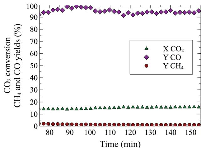
Fig. 3 Reverse water gas shift reaction over 78.3 mg of La<sub>0.75</sub>Sr<sub>0.25</sub>-FeO<sub>3</sub> at 550 °C. Total flow 50 sccm (10% H<sub>2</sub> 10% CO<sub>2</sub> v/v, He balance). Previously, catalyst was reduced for 20 min in 10% H<sub>2</sub>/He at 550 °C.
