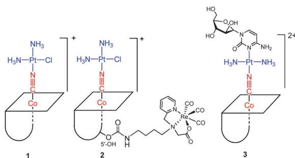
Fig. 2 Structures of B12 derivatives including [{Co}-CN-{*cis*-PtCl(NH<sub>3</sub>)<sub>2</sub>}]<sup>+</sup> (**1**), [{Re}-{Co}-CN-{*cis*-PtCl(NH<sub>3</sub>)<sub>2</sub>}]<sup>+</sup> (**2**), and [{Co}-CN-{*trans*-Pt(Cyt)(NH<sub>3</sub>)<sub>2</sub>}]<sup>2+</sup> (**3**).
