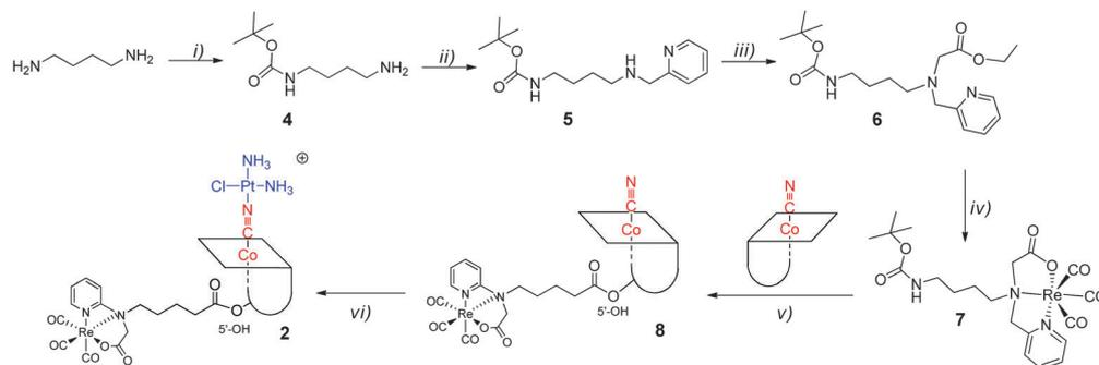
Scheme 1 Synthesis scheme towards [{Re}-{Co}-CN-{*cis*-PtCl(NH<sub>3</sub>)<sub>2</sub>}]<sup>+</sup> (**2**): (i) Boc<sub>2</sub>O; (ii) py-2-CHO, NaBH<sub>4</sub>; (iii) BrCH<sub>2</sub>CO<sub>2</sub>Et; (iv) [NEt<sub>4</sub>]<sub>2</sub>[ReBr<sub>3</sub>(CO)<sub>3</sub>]; (v) TFA and then CDT, TEA; (vi) cisplatin, AgNO<sub>3</sub>.
