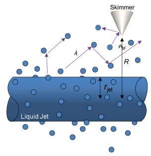
Fig. 4 Evaporating molecules create a vapor cloud surrounding the liquid microjet. The number of vapor-vapor collisions over the distance R depends on both the mean free path  $\lambda$  and the jet radius  $r_{\rm jet}$ .
