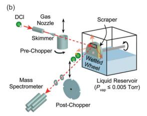
Fig. 3 Experimental setups used in our laboratory for molecular beam scattering experiments with (a) liquid microjets and (b) flat liquid films. The figure illustrates collisions of DCl that exit the liquids as DCl and D  $\rightarrow$  H exchanged HCl.
