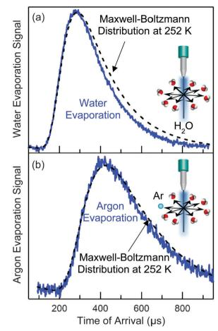
Fig. 5 Time-of-flight (TOF) spectra of (a) water molecules and (b) dissolved argon atoms evaporating from a pure water microjet of radius  $r_{\rm jet} = 5~\mu{\rm m}$ . The best-fit dashed lines are Maxwell–Boltzmann distributions at  $T_{\rm liq} = 252~{\rm K}$ . Adapted with permission from C. Hahn, Z. R. Kann, J. A. Faust, J. L. Skinner and G. M. Nathanson, *J. Chem. Phys.*, 2016, **144**, 044707. Copyright 2016, AIP Publishing LLC.
