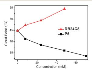
Fig. 4 Supramolecular control over the LCST-type phase behaviour through different macrocyclic compounds. The concentration of IL-I for each measurement is at 500 mg mL<sup>-1</sup>, 2.2 M.
