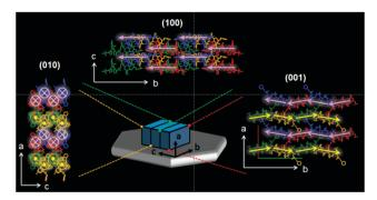
Fig. 4 The complete molecular arrangement of foldecture  $P_1$ . A blue box representing a unit cell is laid on the hexagonal plate (gray) alongside the absolute axes. Extended molecular networks (2  $\times$  2  $\times$  2) as viewed along the a- (top), b- (left), and c-axes (right) show the molecular-level packing. The pink and yellow arrows and symbols ( and ( ) superimposed on each foldamer indicate the helical direction (N to C).
