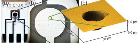
Fig. 1 (a) Photo of the thin-film microarray electrode, (b) optical microscope image of the platinum working electrode, consisting of a platinum disk electrode ( $\mathcal{O}_{Pt\text{-disk}} = 1 \text{ mm}$ ) covered by a (3.0  $\pm$  0.5  $\mu m$  thick) SU-8 layer and defined by 90 microholes ( $\mathcal{O}_{u\text{-hole}} = 10 \mu m$ , pitch = 100  $\mu m$ ), (c) atomic force microscopy (AFM) mapping of a working electrode microhole.
