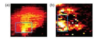
Fig. 6 SERS mapping images of a MCF7 cell expressing HER-2 using hollow gold nanoparticles (a) and silver nanoparticles (b) specific for HER-2 at 1620 cm<sup>-1</sup>, demonstrating the feasibility of using SERS probes for cancer detection. Reproduced, with permission from Elsevier, Copyright 2009, ref. 87.
