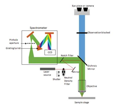
Fig. 2 Standard configuration of a confocal Raman microscope
