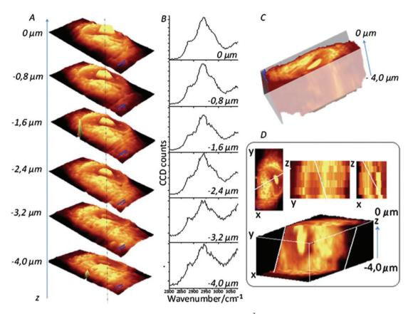
Fig. 7 Confocal Raman imaging-stack of an EA.hy 926 cell covering  $16.7 \times 34.1 \times 4 \, \mu m^3$ . Integration map (A) over the  $\nu_{C-H}$  band (2800–3020 cm<sup>-1</sup> range), single spectra (B) extracted from the same point in the maps (dotted line), a reconstructed 3D image seen from the top (C) and a crosssection of the reconstructed 3D image (D). Reproduced with permission from the Royal Society of Chemistry, Copyright 2013, ref. 99.
