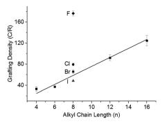
Fig. 4 Grafting density of alkyl halides as a function of alkyl chain length  $(C_nH_{2n+1}Br)$  and halide;  $C_8H_{17}X$  where  $X = F(\spadesuit)$  Cl,  $(\bullet)$ , Br  $(\blacksquare)$ or I (▲) for 20: 1 charged SWCNTs. Line fitted to alkyl bromide series.
