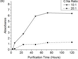
Fig. 6 (a) Concentration of material dissolved versus C/Na after 48 h soaking of 1 mg mL<sup>-1</sup> SWCNT in DMAc. (b) Absorbance (660 nm) of NaNp/DMAc and SWCNTs at a given SWCNT to sodium ratio versus time.
