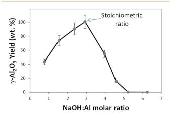
Fig. 3 Effect of the initial NaOH: Al(NO<sub>3</sub>)<sub>3</sub>·9H<sub>2</sub>O molar ratio during hydrothermal synthesis (200 °C, 20 h) on the final  $\gamma$ -Al<sub>2</sub>O<sub>3</sub> yield (wt%).
