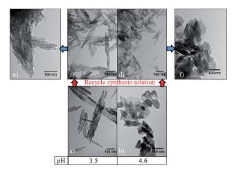
Fig. 4 Initial nanostructured  $\gamma$ -AlOOH hydrothermally synthesised (200 °C, 20 h) at (a) pH 3.5 and (b) 4.6 and morphology of  $\gamma$ -AlOOH synthesised by recycle procedure from initial pH (c) 3.5 and (d) 4.6. (e) and (f) show the morphology of resulting  $\gamma$ -Al<sub>2</sub>O<sub>3</sub> samples after calcination of (c) and (d) respectively.
