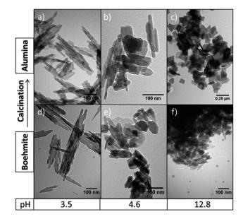
Fig. 1 Effect of pH of the solution on the morphology of  $\gamma$ -Al<sub>2</sub>O<sub>3</sub> (a-c) and  $\gamma$ -AlOOH (d-f) from hydrothermal synthesis (200 °C, 20 h).
