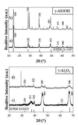
Fig. 5 Assigned X-ray diffraction pattern for  $\gamma$ -AlOOH (a) nanorods and (b) nanoplates synthesised under acidic and basic conditions respectively (200 °C, 20 h) and  $\gamma$ -Al<sub>2</sub>O<sub>3</sub> (c) nanorods and (d) nanoplates. (Acidic = pH 3.5, basic = pH 12.8).
