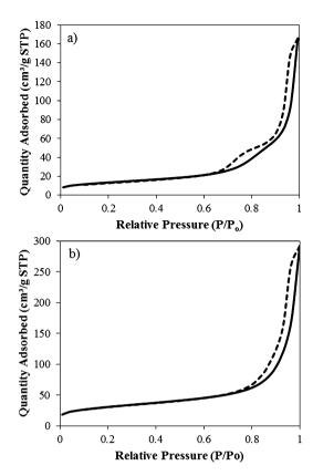
Fig. 6 Nitrogen adsorption—desorption isotherms at  $-196\,^{\circ}\text{C}$  of (a)  $\gamma$ -AlOOH synthesised at 200  $^{\circ}\text{C}$  for 20 h with 1 M NaOH and (b) corresponding  $\gamma$ -Al $_2$ O $_3$  after calcination. (Adsorption = solid line, desorption = dashed line).
