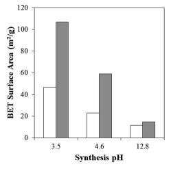
Fig. 7 BET specific surface area for boehmite (white) and alumina (grey) hydrothermally synthesised at pH 3.5, 4.6 and 12.8 for 20 h at  $200\,^{\circ}\text{C}$ .
