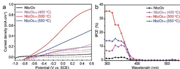
Fig. 4 (a)  $I$ - $V$  curves measured under  $100 \text{ mW cm}^{-2}$  simulated solar light generated by a 100 W xenon lamp coupled with an AM 1.5G filter in 1 M NaOH electrolyte; (b) IPCE spectra measured at 0.2 V vs. SCE in 1 M NaOH electrolyte.
