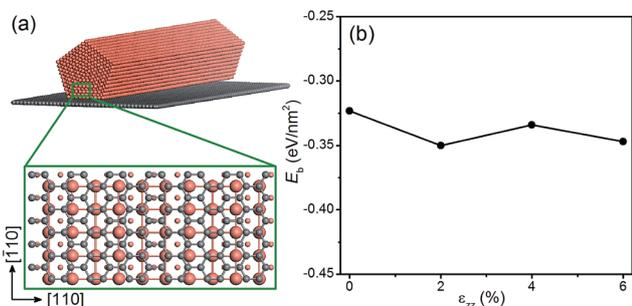
Fig. 8 (a) Schematic of a penta-twinned Cu NW on a graphene substrate. The grey and orange spheres represent C and Cu atoms, respectively. The blown-up view of the DFT supercell is shown in the lower panel. (b) Binding energy of the Cu NW on the graphene as a function of the uniaxial tension.
