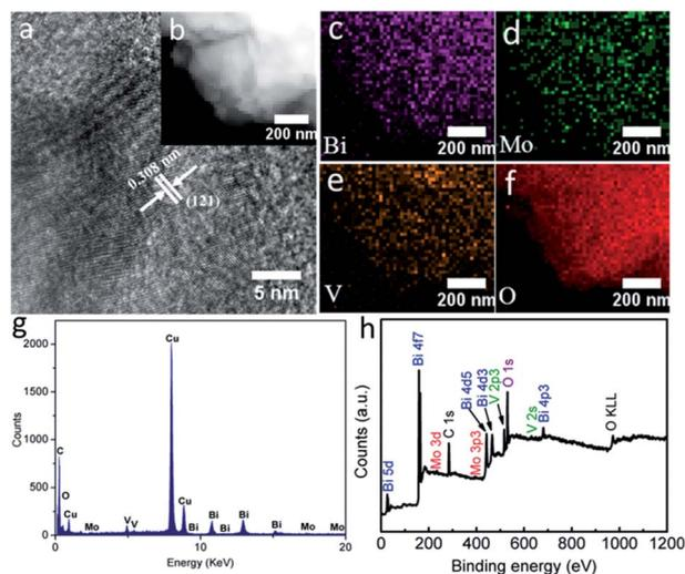
Fig. 3 (a) The HETEM image, (b) HAADF-STEM image, elemental mapping images of (c) Bi, (d) Mo, (e) V and (f) O, (g) EDX spectrum and (h) the survey XPS spectrum of  $\text{BiMo}_{0.015}\text{V}_{0.985}\text{O}_4$ .
