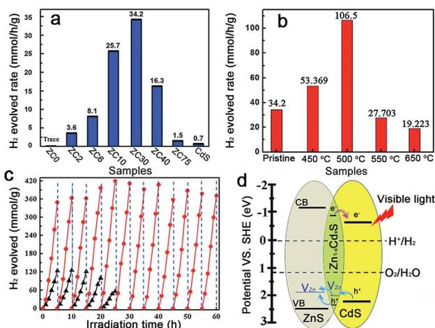
Fig. 3 (a) Photocatalytic H<sub>2</sub>-production activities of the ZCX samples and (b) ZC30 post-annealed at different temperatures in a 0.35 M Na<sub>2</sub>S and 0.25 M Na<sub>2</sub>SO<sub>3</sub> mixed aqueous solution under visible-light irradiation. (c) Comparison of the photocatalytic stabilities of pristine ZC30 (triangle) and ZC30-500 (circle). (d) Schematic illustrating charge transfer and separation in ZnS/Zn<sub>1-x</sub>Cd<sub>x</sub>S/CdS.
