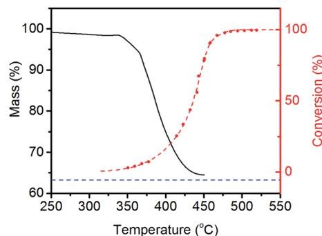
Fig. 4 Thermogravimetric analysis data showing the decomposition of LiNH<sub>2</sub> under ammonia (black), compared with the ammonia decomposition efficiency data under 60 sccm ammonia flow (red) and a sigmoidal fit to the decomposition data (dashed red). The expected mass loss for decomposition to Li<sub>2</sub>NH is shown as a dashed blue line.
