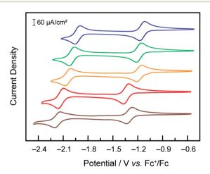
Fig. 1 Cyclic voltammograms under Ar at 50 mV s $^{-1}$  of 1 mM solutions of compounds 1 (— blue), 2 (— green), 3 (— orange), 4 (— red) and 5 (— brown) in DMF, TBAPF $_6$  0.1 M, on a glassy carbon electrode.
