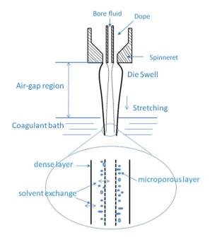
Fig. 21 Schematic diagram of area nearby the spinneret and the formation of nascent hollow fiber during phase inversion.
