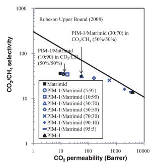
Fig. 19 Comparison with Robeson upper bound of pim-1/Matrimid polymer blends of  $CO_2/CH_4$ .
