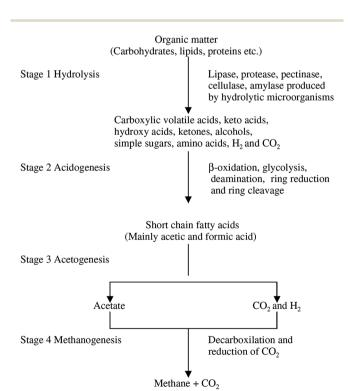
Fig. 3 Metabolic route for the conversion of organic matter to the methanogenic substrates (acetate, CO<sub>2</sub> and H<sub>2</sub>) and finally to CH<sub>4</sub> and CO<sub>2</sub>.
