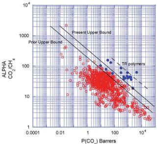
Fig. 8 Robeson upper bound correlation for  $CO_2/CH_4$  separation 2008 (alpha  $CO_2/CH_4$  is selectivity of  $CO_2/CH_4$ ; tr, thermally rearranged data reference).
