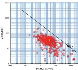
Fig. 17 Correlation of permeability and permselectivity for CO<sub>2</sub>/CH<sub>4</sub> gas pair. The solid line is the Robeson upper bound of 2008. triangles indicate pim-1/zif-8 films after ethanol treatment, squares pim-1/zif-8 films as cast.
