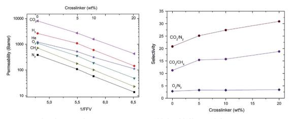
Fig. 16 Permeability of  $N_2$ ,  $CH_4$ ,  $O_2$ , He,  $H_2$ ,  $CO_2$  and gas pair selectivity of  $CO_2/N_2$ ,  $CO_2/CH_4$  and  $O_2/N_2$  in pim-1 and crosslinked pim-1 pegbiazide membranes as 1/FFV and ratio of crosslinker.
