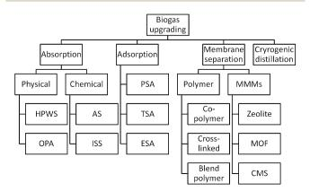
Fig. 4 Current technologies for biogas upgrading.
