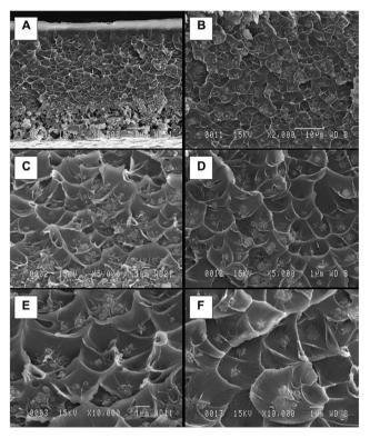
Fig. 11 SEM micrographs of m-zo Matrimid/non-amine-grafted zeolite (a, c and e) and m-IPA-3ET Matrimid/amine-grafted zeolite (b, d and f).
