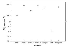
Fig. 33 Annual operation costs splitted in annual operation costs and annual costs for investment (a) and  $CH_4$  recovery for the different hybrid processes at a feed flow rate of 1000 m<sup>3</sup>(STP) h<sup>-1</sup> (b). The  $CH_4$  recovery of the hybrid combined heat and power process (CHP) is significantly lower compared to the other process configuration.
