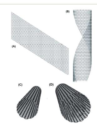
Fig. 12 (a) Flat sheet of graphite, (b) partially rolled sheet of graphite, (c) SWCNTs and (d) MWCNTs.
