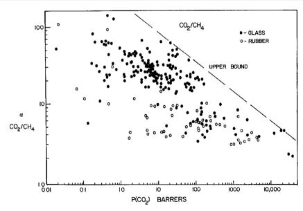
Fig. 7 Literature data for CO<sub>2</sub>/CH<sub>4</sub> ideal selectivity versus CO<sub>2</sub> permeability (1991).
