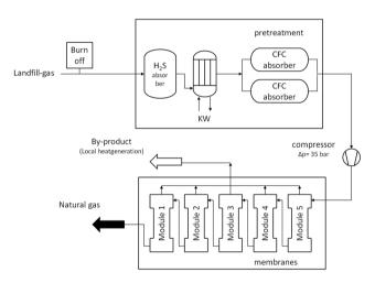
Fig. 29 Flow chart diagram of the pilot plant.
