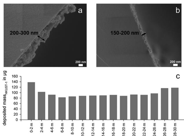
**Fig. 2** Characterization of the HKUST-1 capillary coatings. A – SEM-image of material near the capillary inlet. B – SEM-image of material near the capillary outlet. C – Profile of the mass of deposited HKUST-1 material along the capillary as indicator of the corresponding film thickness variations of the stationary phase.
